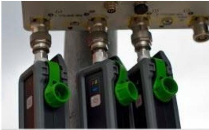
Cable loss can be measured either as a 1-port measurement, with the far end of the cable terminated in an open or short circuit, or directly measured for increased accuracy as a 2-port measurement using a second iVA
