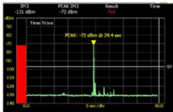
Dynamic testing identifies loose metal-to-metal connections as well as contact surface defects that might cause arcing at higher power levels. Without dynamic testing these defects could go unnoticed until activated by wind loading, tower vibration or stresses caused by temperature changes.
